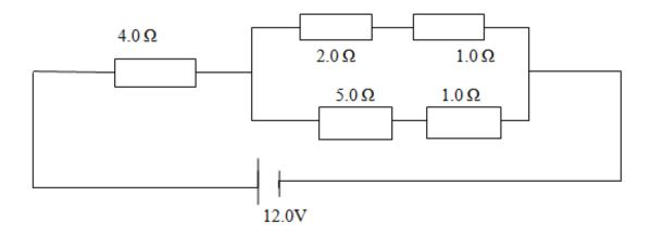
Determine the power dissipated in the 2.0  $\Omega$  resistor in the circuit above (Resistive dissipation)
