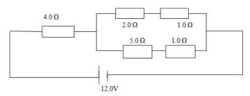
Q2. Determine the power dissipated in the 2.0  $\Omega$  resistor in the circuit above (Resistive dissipation)
