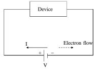
The ratio V/I is a constant, where V is the voltage applied across a piece of material (device) such as a wire and I is the resulting current through the material.
